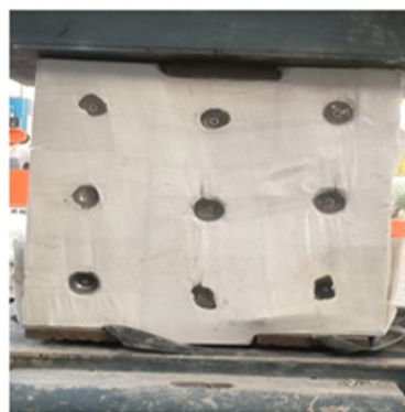
(d) The overall damage of ZTY masonry
