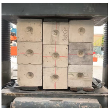
(c) The overall damage of ZT masonry
