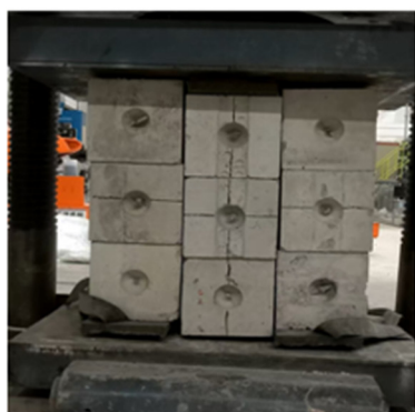
(a) The overall damage of ZS masonry
