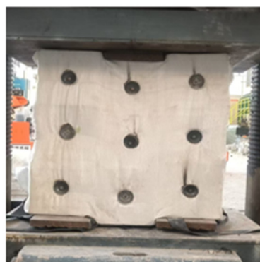
(b) The overall damage of ZYS masonry
