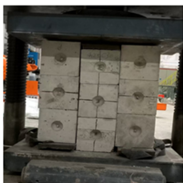
(e) The overall damage of ZST masonry
