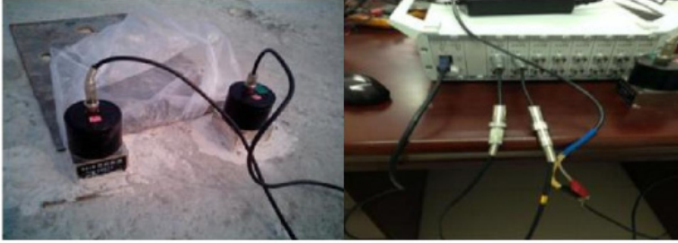
Fig. 14. Main Girder Amplitude Sensor
