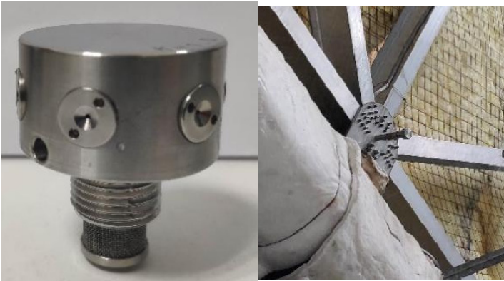
(a) Special spray nozzle and its installation method
