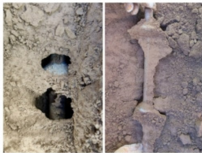
Fig. 8. Failure phenomenon of the soil around the expansion plate
