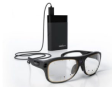
Fig. 4. Tobii Pro Glasses 3 Eye Tracker (Image source: Online, https://www.tobii.cn/products/eye-trackers/wearables/tobii-pro-glasses-3 )
