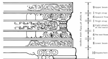
Fig. 1. Schematic diagram of the composition of the Sumeru pedestal
