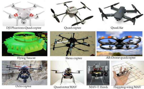
Fig. 1. UAVs with different structural designs [4]
