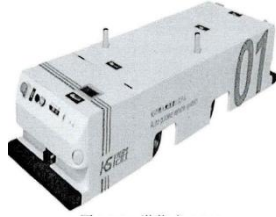
Fig. 2. Latent traction structure AGV [7]
