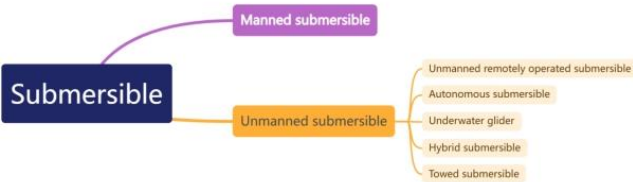
Fig. 2. Classification of submersibles division based on manned and unmanned [2]
