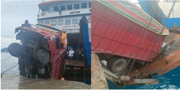
Figure 1. Ramp door MV Watunapato broken Source : manado.tribunnews.com
