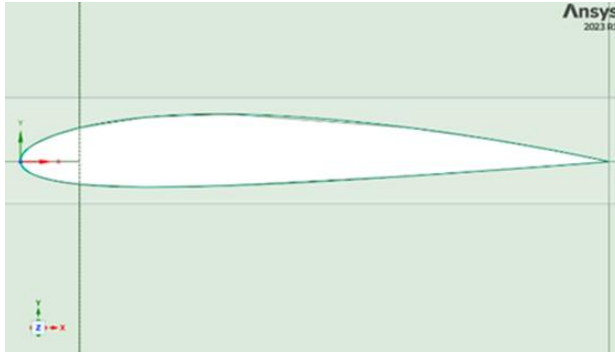
Fig. 2. Detailed close-up NACA2412 airfoil (Picture credit: Original)
