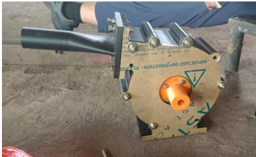
Figure 5. Assembly Cross-Flow Turbine Components
