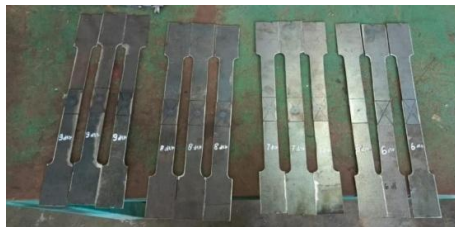
Figure 6. Preparation of Tensile Test Specimens
