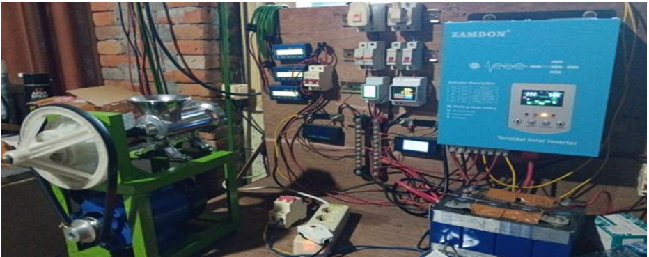
Figure 3. Energy Measurement Circuit for Spice and Meat Grinding Machine
