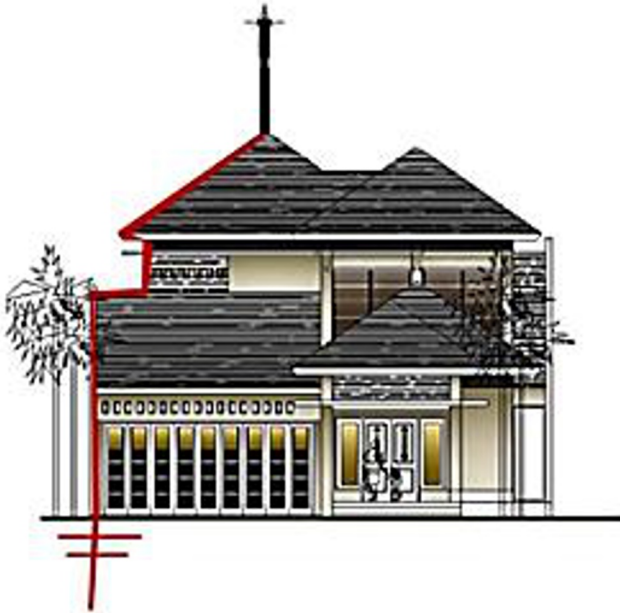
Figure 4. Illustration of the Installation of an Electrostatic Lightning Rod
