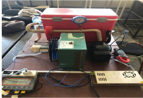
Figure 3. The Prototype Product is a Solar-Powered Vapor Compression Mini Cooler for Fish Storage with a Cooling Capacity of 1/8 PK
