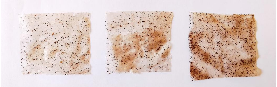
Figure 1. Bioplastic Films with 10%, 20%, and 30% Spent Coffee Grounds Content (Left to Right).
