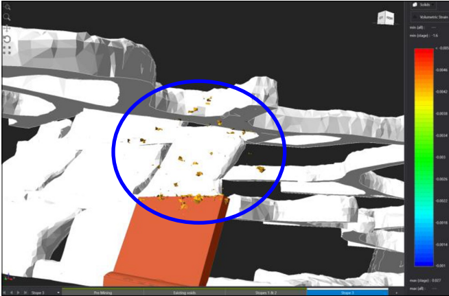
Figure 13 Isosurfaces (orange) representing damage (cracking) at a SRF of 2.0
