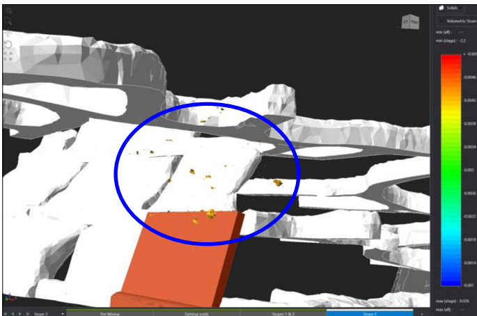
Figure 12 Isosurfaces (orange) representing damage (cracking) at a SRF of 1.0
