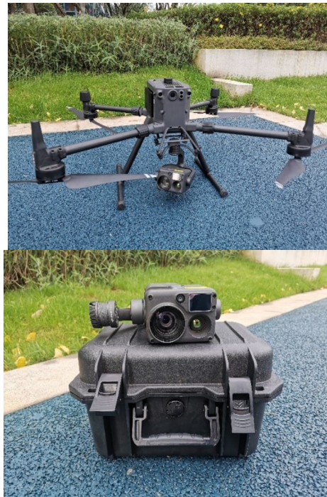
Fig. 1. DJI Matrice 300 RTK UAV (left) and DJI Zenmuse XT2 camera with twin-lens of RGB and thermal infrared (right)
