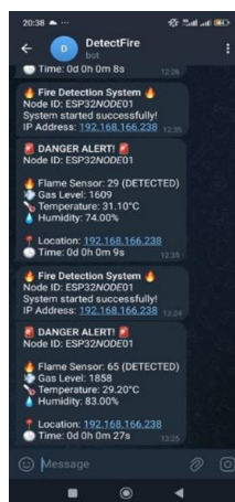
Fig. 6. Example of a Telegram notification sent by the proposed IoT-based fire detection system, showing hazard type, timestamp, and location details as received by users during testing.
