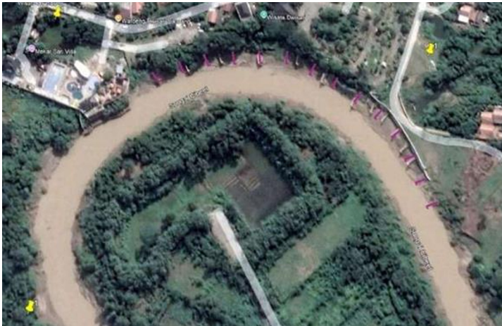
Fig. 10. Proposed placement of 14 groynes at the bend of the cibeeet river, marked in pink.
