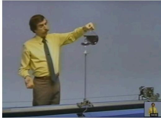
Fig. 2. Inverted Pendulum Demonstration with a Cup on Top of Pendulum(MIT OpenCourseWare).
