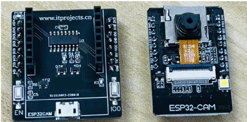
Fig. 4. ESP32-CAM layered motherboard used in the car.
