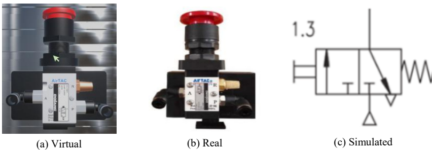
Fig. 2. 3D Realistic Models of: virtual 3/2 pneumatic valve in VL-MN (a), real 3/2 pneumatic valve in Real-MN (b), and symbol of 3/2 pneumatic valve in FluidSIM (c).
