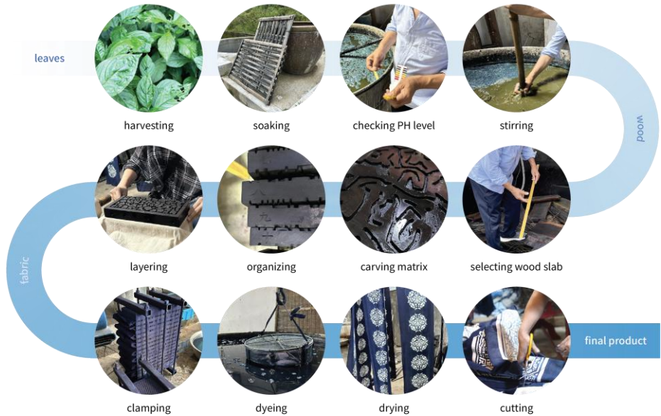
Fig. 1. The process for producing indigo-dyed fabrics, from leaf harvesting to the finished product. The figure illustrates the method employed in Wenzhou, which resembles processes used in other geographical areas.
