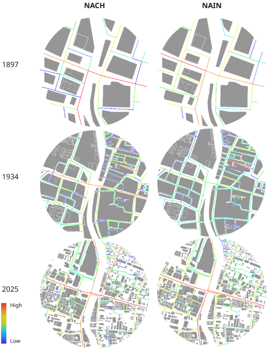
Fig 7. Surabaya Normalised Integration (NAIN) and Normalised Choice (NACH) in the years 1897, 1934, and 2025
