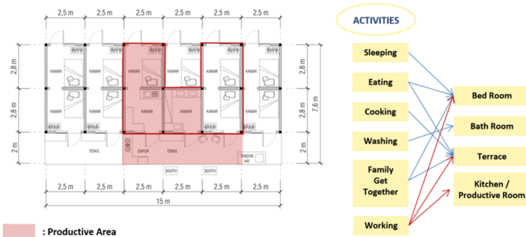
Figure 7. The floor plan of the Mixed Cake Houses – Mrs. Ruli explains the domestic and productive areas, as well as the rooms used for conducting both domestic and productive activities.
