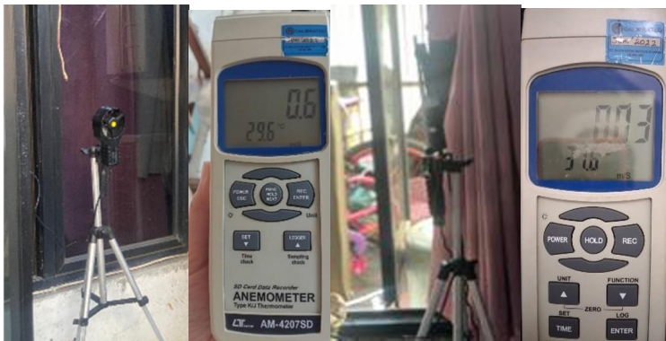
Fig. 1. (a) Anemometer Sensor Position, and the data recorder, (b) Anemometer Hotwire Sensor Position and the data recorder
