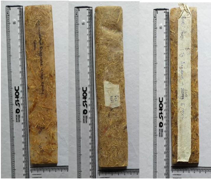
Fig.2. Samples with ratio 14:1, 11:1, 8:1
