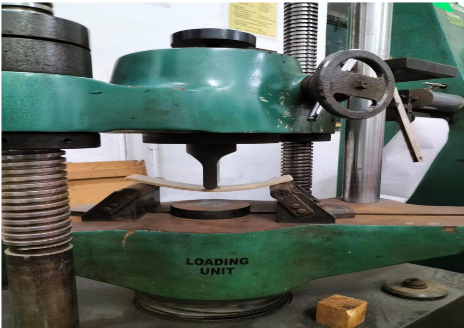
Fig.3. Flexural Strength Testing Set Up
