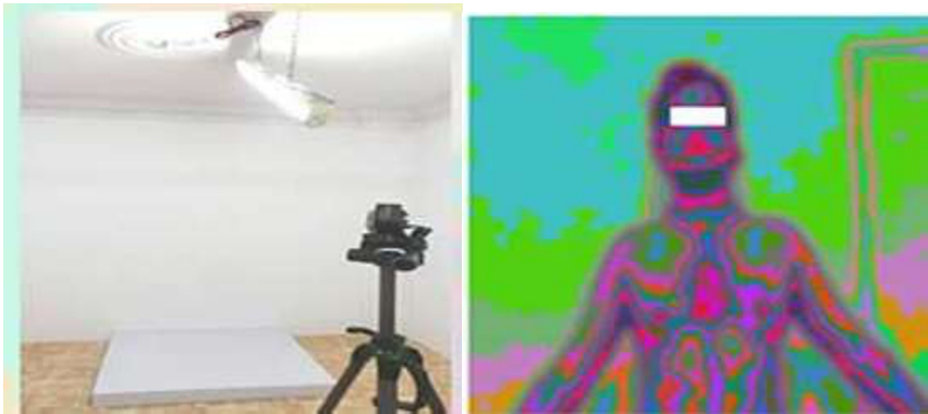
Figure (3a) Setup and (3b) image of Polycontrast Interference Photography [21]
