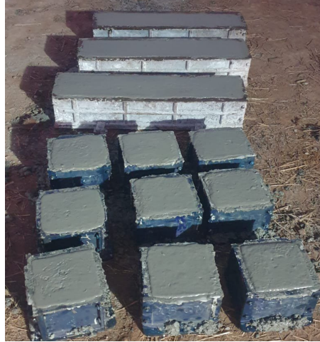
Fig. 8 Concrete cube casted for compressive strength testing for 3, 28 & 56 day.
