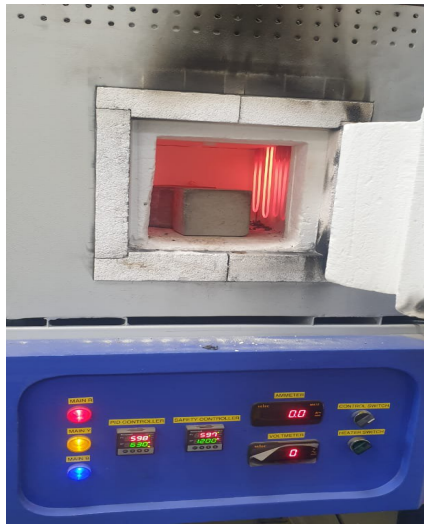
Fig. 11 Furnace 1450°C for high temperature cube testing.
