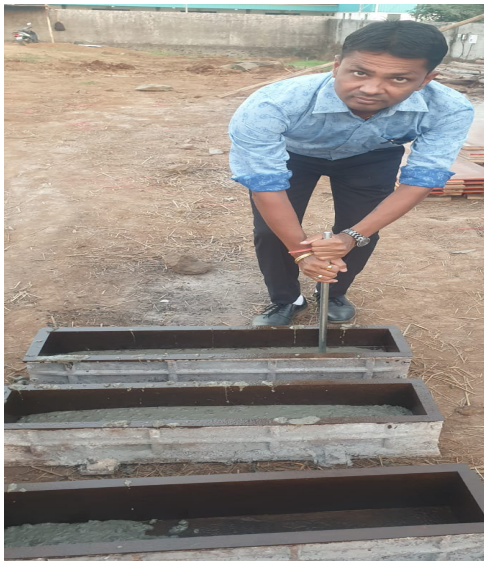
Fig. 7 Beam and Cube casting for compressive strength testing.
