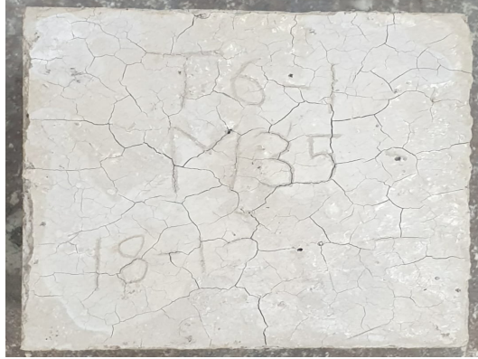
Fig. 12 Crack on cube after heating at 650°C.
