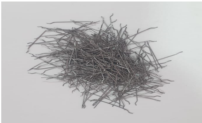
Fig. 17 Steel Hook fibre of Diameter 1 mm.
