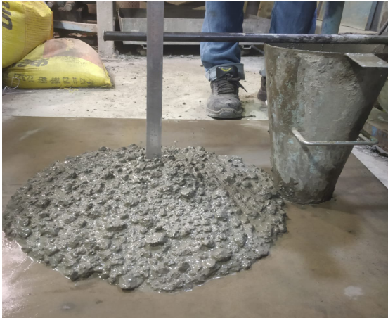
Fig. 6 120 minute's slump flow 220 MM.
