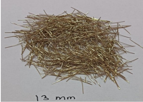
Fig. 15 Brass Coated Steel fibre of Diameter Avg. 0.3 mm.
