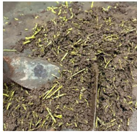
Fig 5. Raw mix with Polypropylene fibers
