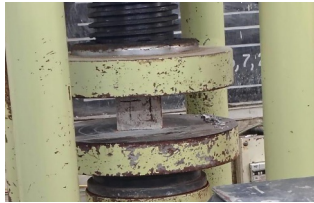
Fig 3. Compressive strength testing at 28 days
