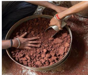
Fig 1. Crushing of waste bricks into a fine powder
