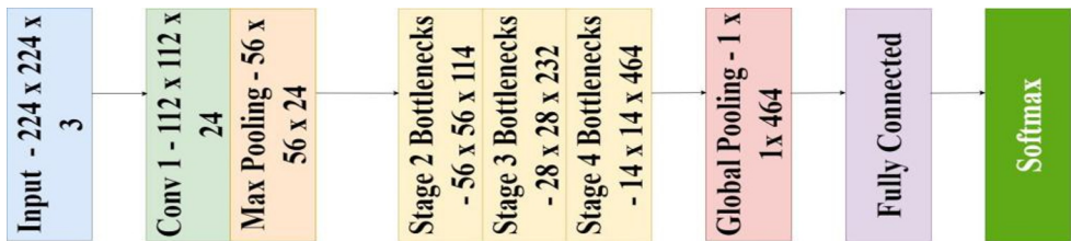
Fig. 2. Principles Behind ShuffleNet v2 Architecture
