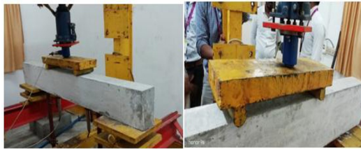
Fig.5 Control beam (flexure) testing under four-point bending
