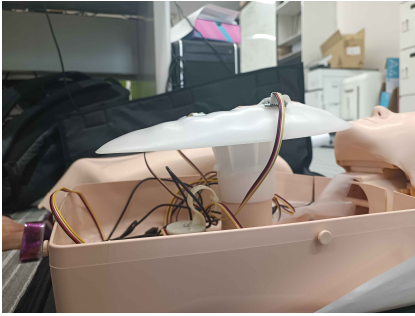
Fig. 3. Manikin's internal configuration (side view). In the actual BLS training, this body is covered with a vinyl cover that simulates the texture of human skin (the cover can be seen in the left side in Fig.4). The Raspberry Pi under the chest cannot be seen (not seen in Fig.4, too).
