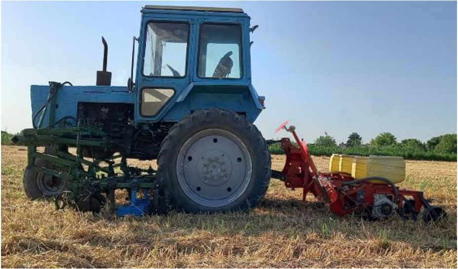
Figure 3. Drawing. A combined unit for minimal tillage in wheat-free fields and for sowing seeds of repeated crops.
