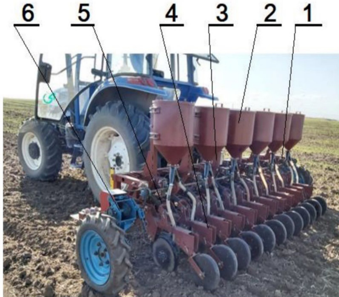
Figure 1. A seed drill based on No-till technology, developed for the soils of Northern Kazakhstan. 1-frame, 2-seed hopper, 3-application device (fertilizers), 4-sowing section, 5-sowing machine, 6-drive wheel (movement wheel)
