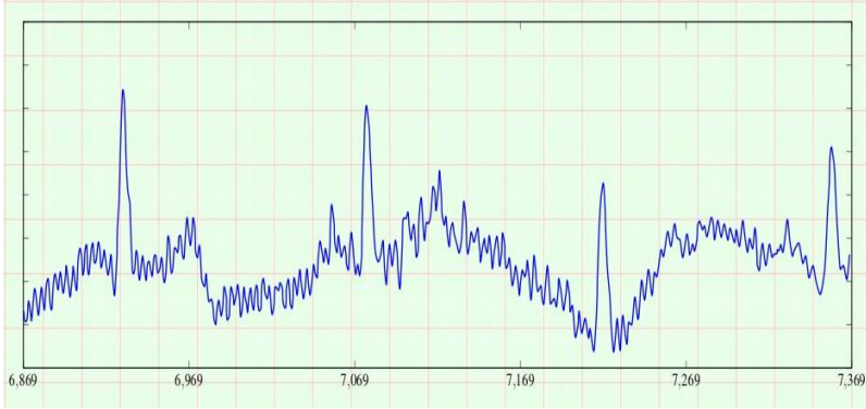
Fig. 6. Raw ECG Signal Data of Arduino IDE Serial Plotter.
