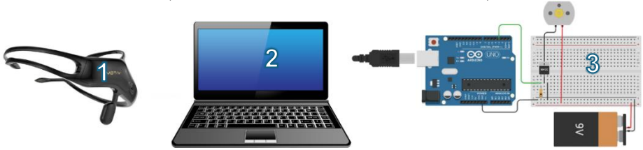
Figure 1. The hardware design of the EEG-BCI-based system for controlling a DC motor
