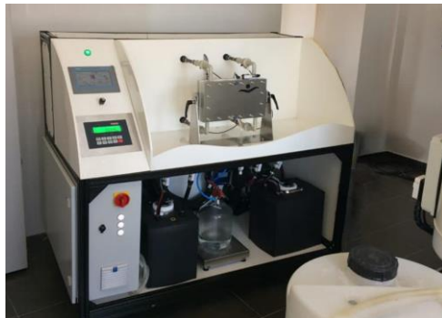
Fig 2. Photograph of the laboratory-scale AGMD experimental unit used at the PURA-Lab, Plataforma Solar de Almería (PSA).
