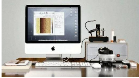
Fig. 1 The Nanoeducator microscope, operating based on the atomic force microscopy principle.
