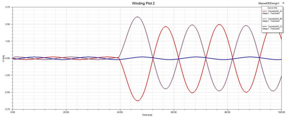
Fig. 10. Low-Voltage Side Phase Current in Phase-Phase Fault
