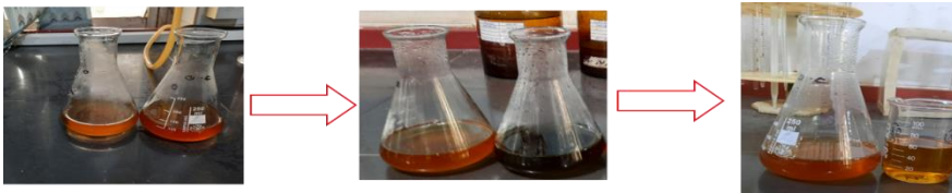
Fig. 2. The sequence of steps in the decolorization phase using ozonation and activated carbon.
