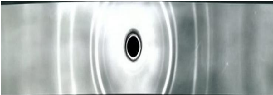
Fig.1. Debye diffraction pattern of p-type \text{Cu}_2\text{O} thin films prepared by chemical deposition method
