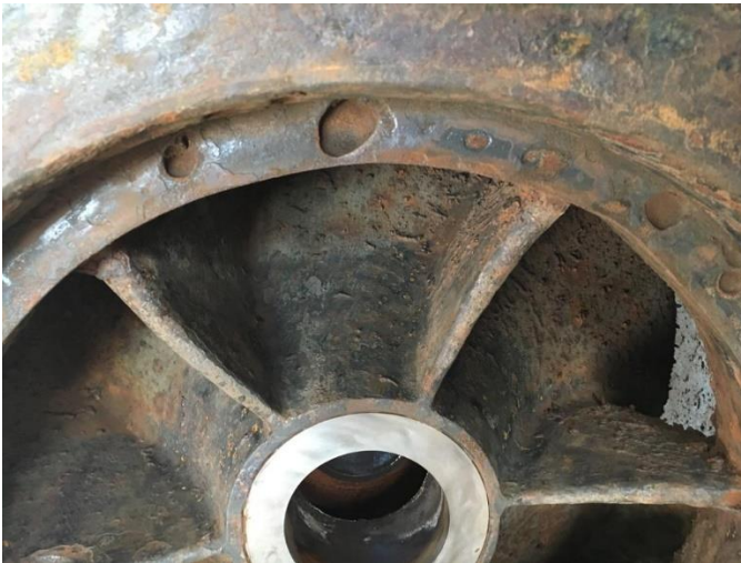
Fig. 3. Severe Erosion-Corrosion on Pump Components
