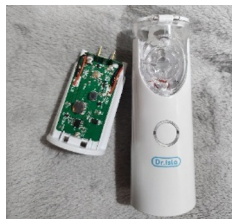
Fig.8. Frame and PCB of Dr.Isla portable nebulizer Model-N6
