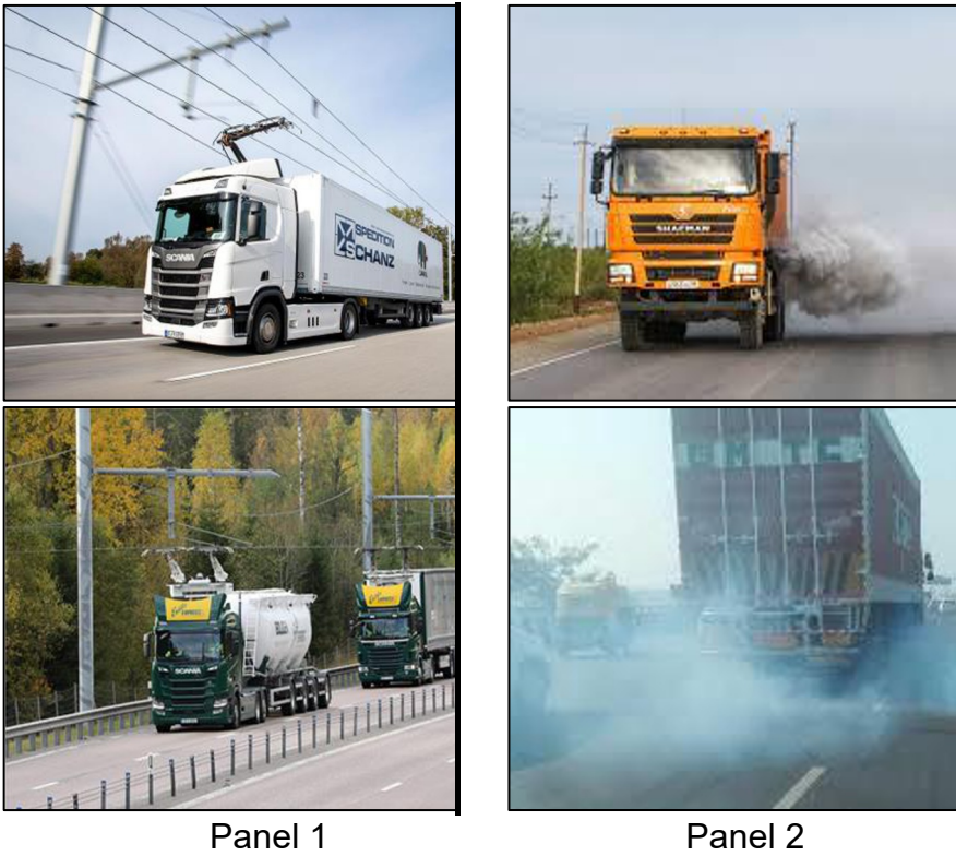
Fig.2. Panel 1 (left) illustrates hybrid e-trucks equipped with pantographs operating in zero-emission mode along an electrified corridor. Panel 2 (right) shows conventional diesel trucks emitting pollutants from the tailpipe during freight transport.
