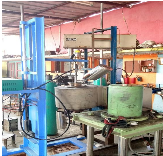
Fig. 1. Ultrasonic Cavitation assisted casting technique setup
