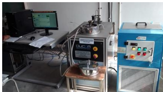
Fig. 2. High temperatures Tribometer pin on disc: DUCUM Make
