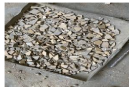
(b) Ceramic tile aggregate (CT)
