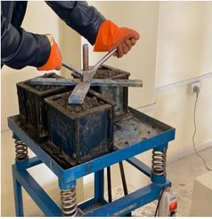
Fig. 3: Compaction by vibration
