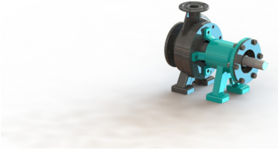
Fig. 2. 3D model of a centrifugal pump after assembly.
